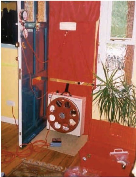
Typical domestic pressure testing equipment
